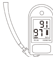
Figure 6. Mounting the lanyard
